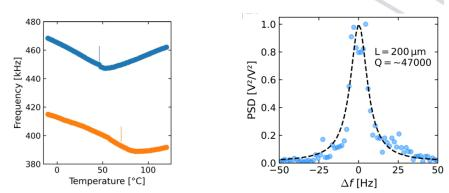
(left) Array of microbridge resonators made of 100nm-thick LSMO deposited on  $SrTiO_3(110)$  substrate.(center) Temperature dependence of the resonance frequency of LSMO bridge resonators showing the effect of the magnetic transition on the mechanical response (Curie temperature is marked by arrows). (right) Spectral response of a 250µm-long LSMO bridge, mechanical quality factor is obtained form Lorentzian fit.
