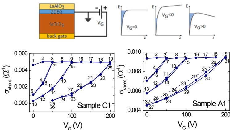
Fig. 1: Top: Sketches of the two dimensional electron gas (2DEG) at the interface and circuitual configuration. Bottom: Zero field longitudinal conductance  $\sigma_{\text{sheet}}$  of crystalline (C1) and amorphous (A1) samples as a function of applied gate voltage  $V_G$ , in successive  $V_G$  ramps from zero to  $V_{G\text{max}}^{(i)}$ , with increasing values  $V_{G\text{max}}^{(i)}$ , measured at 20 K.
