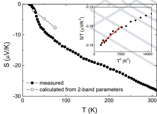
Fig. 2: Measured Seebeck coefficient of LaFe<sub>2</sub>As<sub>2</sub> (filled symbols). The diffusive contribution to the Seebeck coefficient, calculated from the two-band parameters, is also shown in the main panel (open symbols). Inset:  $S/T$  versus  $T^2$  plot, with a linear regime identified in correspondence of the temperature range 40-85 K, which identifies the phonon drag Seebeck coefficient, related to the large electron-phonon coupling.
