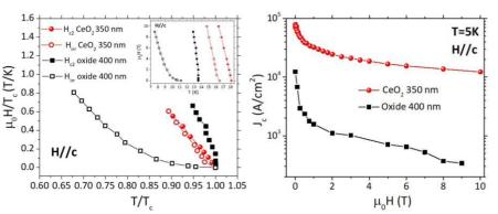
Fig. 2: J<sub>c</sub> at 5 K vs applied magnetic field of the 11 thin films deposited on Hastelloy substrate with 400 nm of oxide (black) and on the RABiT substrate with a 350 nm thick CeO<sub>2</sub> buffer layer (red).
