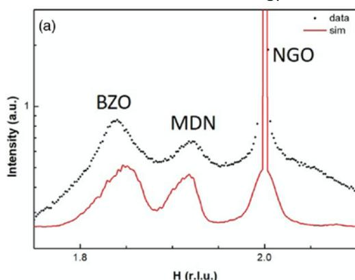
Fig. 1: Surface x-ray diffraction intensity scans along the H direction of a 2.9-nm BZO film on NGO. The full red lines represent theoretical simulations of the diffraction experimental data. BZO, NGO, and MDN tags specify the diffraction peaks associated to the film, to the substrate, and to the misfit dislocation network, respectively.
