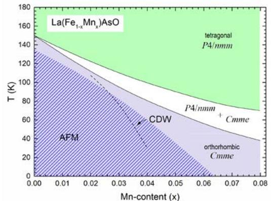
Fig. 2: Phase diagram of the  $\text{La}(\text{Fe}_{1-x}\text{Mn}_x)\text{AsO}$  system (Mn-poor side); the hatched area represents the region of the phase diagram where long-range magnetic ordering takes place; the dotted line defines the region where a static CDW state was detected.
