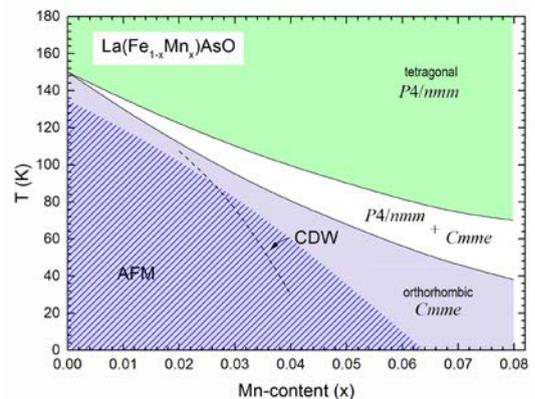
Fig. 2: Phase diagram of the La(Fe<sub>1-x</sub>Mn<sub>x</sub>)AsO system (Mn-poor side); the hatched area represents the region of the phase diagram where long-range magnetic ordering takes place; the dotted line defines the region where a static CDW state was detected.
