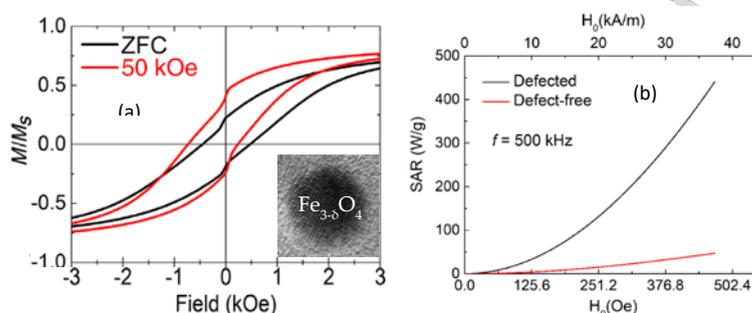
Fig. 2: (a) Normalized hysteresis loops at 5 K for the single-phase spherical nanoparticles taken under zero- and field-cooled ( $H_{\text{cool}} = 50$  kOe) protocols, (b) Monte Carlo calculation of SAR (specific adsorption rate) values as a function of the AC field amplitude,  $H_0$ , at a field frequency  $f = 500$  kHz.
