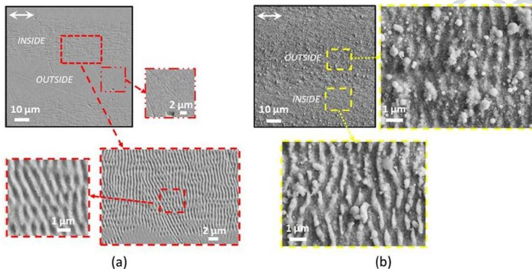
Fig. 1: SEM images of the sample surface addressing the morphological features for a peak fluence of: (a)  $F_p = 0.8 \text{ J/cm}^2$ ; (b)  $F_p = 6.5 \text{ J/cm}^2$ . The SEM images within the dashed boxes are zoomed views of the selected areas. The double-headed arrow indicates the laser beam polarization.
