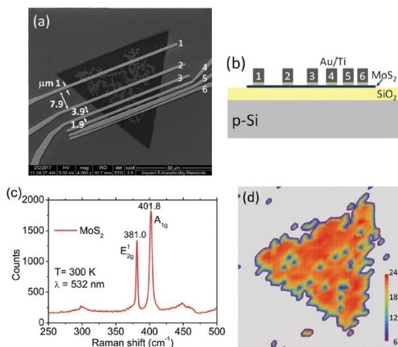
Fig. 1: a) SEM top view of a CVD-synthesized bilayer MoS<sub>2</sub> with Ti/Au contacts. b) Schematic of the back-gate transistors. c) Raman spectrum of the bilayer MoS<sub>2</sub>. d) Map of the difference between A<sub>1g</sub> and E<sub>2g</sub> peaks of micro-Raman spectra.
