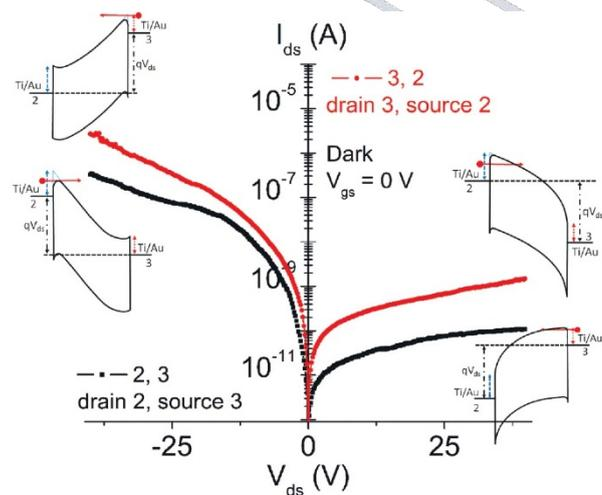
Fig. 2: Band diagram based on two back-to-back Schottky barriers. The forward current for negative V<sub>ds</sub> is due to the image force barrier lowering at the forced junction, while the lower (reverse) current at V<sub>ds</sub> > 0 V is limited by the low electric field at the grounded junction.
