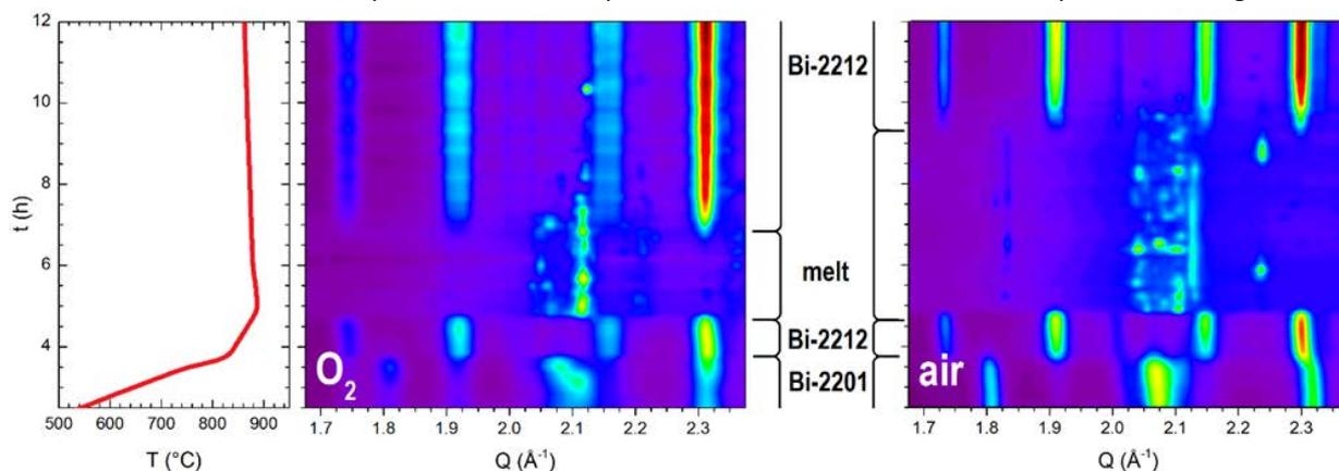
Fig. 1: Phase evolution in the multifilamentary wires during the first 12 hours of the thermal treatment in  $O_2$  (on the left) and air (on the right).
