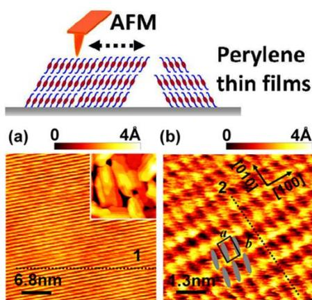
Fig.1: (a) Topography of a PDI8-CN<sub>2</sub> monomolecular terrace revealing an ordered, rippled surface. In the inset, a large-scale morphology (1.5 × 1.5 μm<sup>2</sup>) shows connected mesalike grains forming the polycrystalline thin film. (b) High-resolution topography of the periodic surface structure, with superimposed the anisotropic ab unit cell. Ellipses indicate the orientation of the alkyl chains predicted by a bulk structural model.
