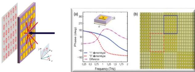
Fig. 1: Diffuse scattering on a coding metasurface under normally incident plane wave illumination (left) is realized exploiting the phase difference ( $0/\pi$ ) (right, (a)) between two types of "supercell" (right, (b)).
