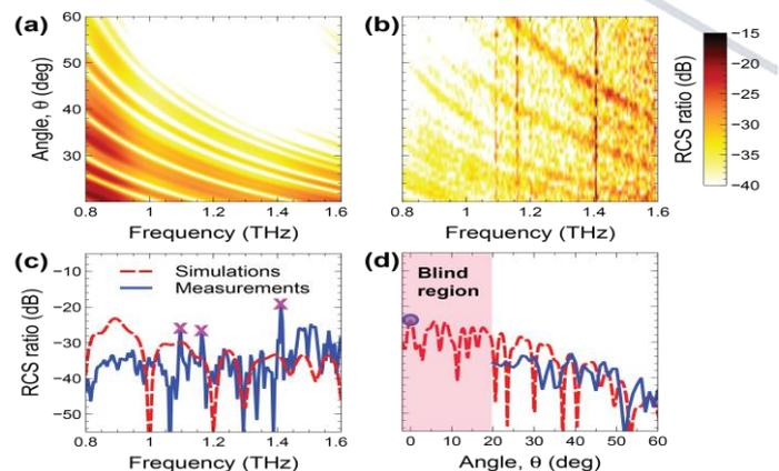
Fig. 2: Normalized Radar Cross Section (RCS) for normal-incidence simulated (a) and measured (b) in false-color scale as a function of frequency  $f$  and observation angle  $\theta$ ; RCS vs  $f$  (c) @30° and vs  $\theta$  (d) @1 THz.
