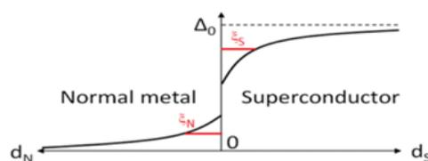
Fig.2: Left: Temperature dependence of normalized  $J_c$ , compared to predictions of models for proximity effect at grain boundary weak links, for different values of the ratio  $d_N/x_N$ . Right: sketch of the proximity effect, illustrating the meaning of the parameters  $d_N$  (thickness of the normal layer) and  $x_N$  (coherence length of the normal layer).
