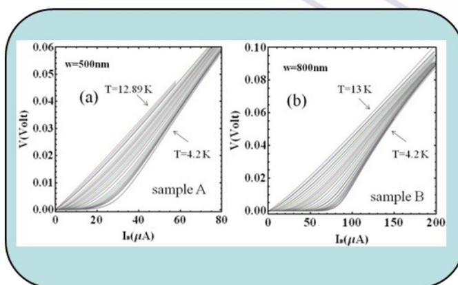
Fig.2: Current voltage characteristics of the nanostrips in the indicated range of temperatures. (a) Sample A,  $w=500\text{nm}$ . (b) Sample B,  $w=800\text{nm}$ . Both samples were  $3\mu\text{m}$  long.
