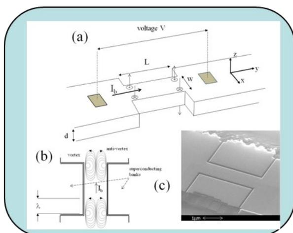
Fig.1: (a) Geometry of the nanostrips used in the work. (b) Schematic of the streamlines of the vortex and anti-vortex current densities. (c) A SEM image of sample B ( $w=800\text{nm}$ ).
