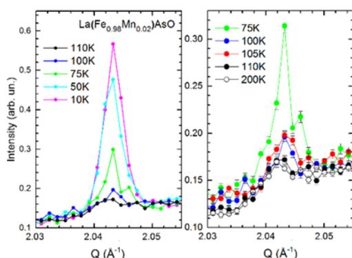
Fig.1: Thermal evolution of the 1<sup>st</sup> order satellite peak of La(Fe<sub>0.98</sub>Mn<sub>0.02</sub>)AsO, marking the occurrence of the CDW state.
