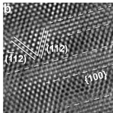
Fig.2: HRTEM image of La(Fe<sub>0.98</sub>Mn<sub>0.02</sub>)AsO phase at 94 K evidencing structural modulation.
