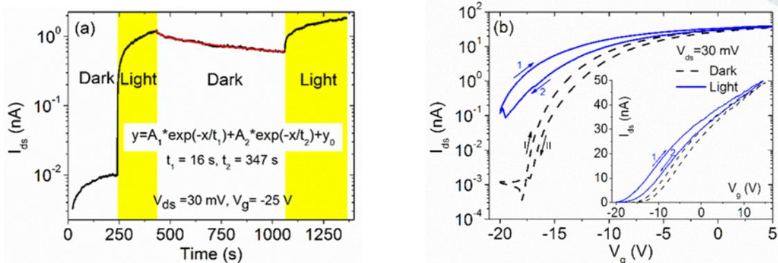
Fig.1: (a) Channel current versus time with and without light. (b) Comparison of transfer characteristics in dark and under illumination (the inset shows the current in linear scale).
