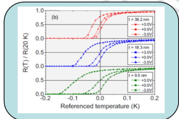
Fig.2: Effect of a gate voltage  $V_G = \pm 3$  V on the  $R(T)/R(20\text{ K})$  vs  $T$  curves for three values of thickness: 39.2, 18.3, and 9.5 nm. The referenced temperature is defined as  $T^* = [T - T_c^{\text{ref}}]_{V_G} - [T_c^{\text{active}} - T_c^{\text{ref}}]_0$ .
