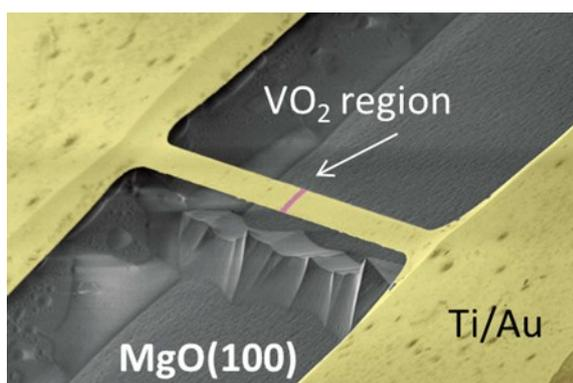
Fig.1: False-colored scanning electron microscopy picture of a microbridge. Electrical current is injected by the gold pads (yellow) into the VO<sub>2</sub> region (magenta). The phase transition is triggered by the temperature increase due to Joule effect.
