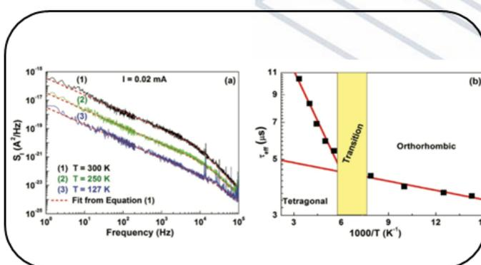
Fig.2: (a) Noise spectra of a perovskite photovoltaic device. (b) Arrhenius plot of the effective lifetime coefficient  $\tau_{\text{eff}}$ . Two distinct behaviors are observed in the tetragonal and orthorhombic phases of the perovskite.
