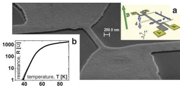
Figure 1. S.E.M. image of a 230 nm wide YBCO bridge. Inset a) shows the scheme of the magnetoresistance setup, inset (b) shows the log-linear plot of the bridge resistance in the temperature range (30–90) K.
