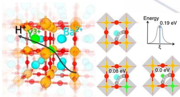
Figure 2. (Left) BZY lattice with the relaxed atomic positions as obtained from a DFT calculation. (Right) Proton transfer between two nearest neighbor O<sub>2</sub><sup>-</sup> ions coordinated or in close proximity of substitutional Y dopants, together with a schematics of the energy profile visited during the proton transfer process. The energy barrier values calculated by DFT are also shown in each panel.
