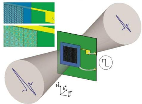
Figure 2. Sketch of the experimental set-up used to test the tunability of the metamaterial response.
