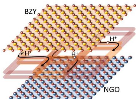
Schematic drawing of the interface between BZY film and NGO substrate with the dislocation network as fast pathway for proton conduction.
