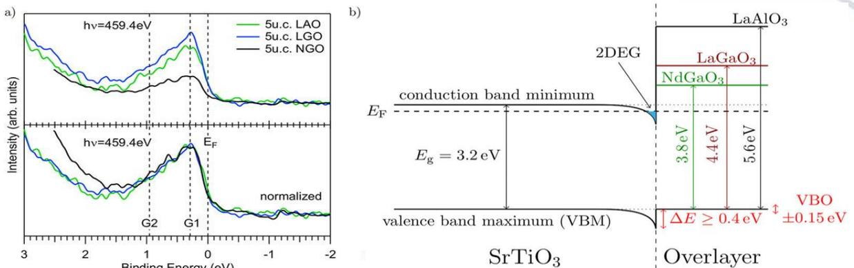
Left image: Resonant photoemission on the Ti 3+ states of the Ti L-edge. The presence of states at the Fermi level, with similar spectral shape, is seen for all samples. Right image: band diagrams are derived from our data.
