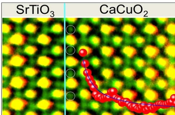
Figure: STEM image of the  $\text{CaCuO}_2/\text{SrTiO}_3$  interface. The white circles indicate the excess oxygen ions at the interface Ca plane. The red bullets indicate the holes concentration decay on going far from the interface with  $\text{SrTiO}_3$ .
