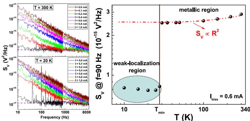
(Left) The spectral traces in the metallic (300 K) and WL (20 K) regions are shown for a 12 nm ultrathin copper film. (Right) Its noise amplitude, at 90 Hz and at a fixed bias current of 0.6 mA, is reported as a function of temperature.
