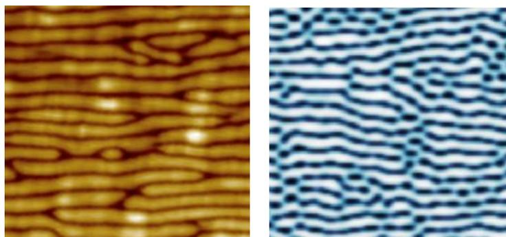
*Atomic Force microscopy image of the reorganized polymer morphology (left) and simulation (right) after exposure to light*
