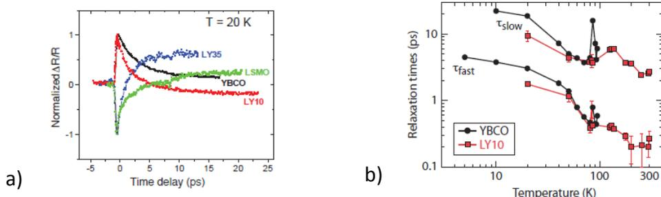
a) Normalized  $\Delta R/R$  transients versus time delay measured at 20 K for our LY10 and LY35 bilayers, as well as the pure YBCO and LSMO reference samples. b) Characteristic fast and slow relaxation times ( $\tau_{\text{fast}}$  and  $\tau_{\text{slow}}$ ) extracted from the experimental  $\Delta R/R(t)$  plots for our LY10 and pure YBCO samples as a function of temperature.
