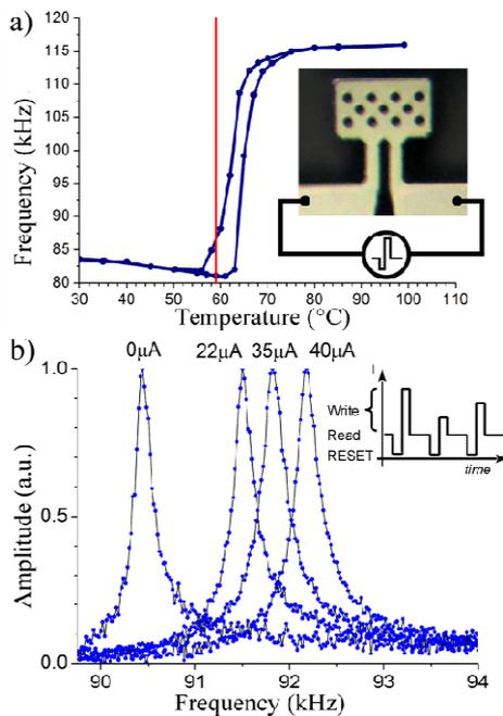
Fig.: a) Temperature dependence of the first flexural mode of the (unbiased) VO<sub>2</sub> microcantilever. b) Mechanical resonances of the microcantilever measured within the hysteretic windows (59 °C) and 15 μA constant read current bias upon a series of erase (0 μA)/write (22-35-40 μA) pulses (inset).
