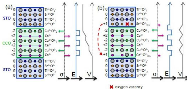
**Fig.1** Sketch of CCO/STO SLs. (a) Unreconstructed interfaces with the diverging electrostatic potential. (b) Reconstructed interfaces by oxygen redistribution in the alkaline-earth metal interface planes.
