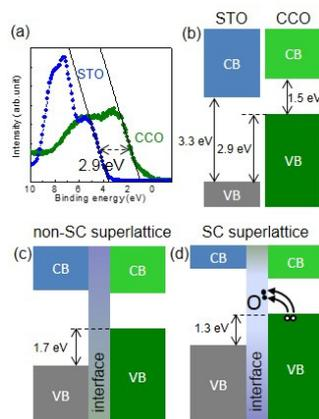
**Fig.2** (a) Valence-band spectra for the CCO and the STO. (b)–(d) Schematic diagram of the valence and conducting bands: (b) uncoupled CCO and STO, (c) non-SC SL and (d) SC SL.
