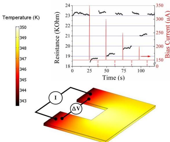
Temperature distribution calculated on a VO<sub>2</sub>/TiO<sub>2</sub> cantilever under 100 µA bias current. Sample temperature is fixed at 343 K and multi-resistance states written by current pulses of different magnitude, cantilever is powered with 150 µA current bias. Erasing is possible by a short pulse to zero. Adapted from L. Pellegrino et al. *Adv. Mater.* 24 2929-2934 (2012).
