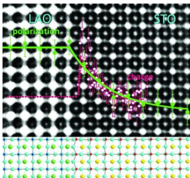
Using state-of-the-art, aberration-corrected scanning transmission electron microscopy and electron energy loss spectroscopy with atomic-scale spatial resolution, experimental evidence for an intrinsic electronic reconstruction at the LAO/STO interface is shown. We demonstrate that in a highly perfect interface, where cation intermixing is negligible, the lattice polarization and the amount of injected charge are in agreement with the predictions of the ER model.
