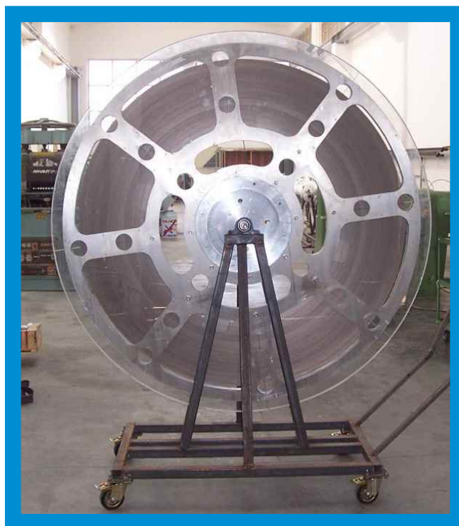
1.6 Km length multifilamentary superconducting MgB 2 wire made in SPIN
