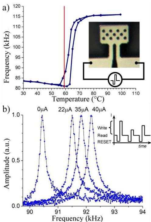
Fig.: a) Temperature dependence of the first flexural mode of the (unbiased) VO<sub>2</sub> microcantilever. b) Mechanical resonances of the microcantilever measured within the hysteretic windows (59 °C) and 15 μA constant read current bias upon a series of erase (0 μA)/write (22-35-40 μA) pulses (inset).
