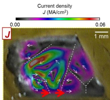
Local Critical Current Density at 5 K in polycrystalline  $\text{FeTe}_{0.5}\text{Se}_{0.5}$  sample (CNR) evaluated by Hall Probe Microscopy (Khyushu University)
