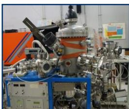
*Pulsed laser Deposition system with in-situ RHEED Diagnostics equipped with a multitarget system for oxide heterostructures and superlattices deposition in oxygen deposition atmosphere enriched with 12% of ozone.*
