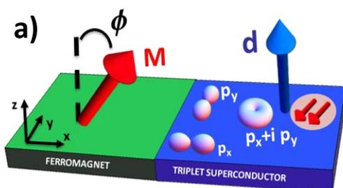
Fig. a) Schematic diagram of the two-dimensional TSC-FM junction. The magnetization  $M$  of the FM can form an angle  $\Phi$  with respect to the  $d$ -vector of the TSC. We study TSC states with  $p_x$ ,  $p_y$ , and  $p_x+ip_y$  orbital symmetry.
