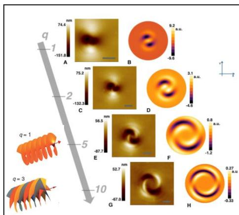
Fig.1 Spiral relief patterns on the surface of azobenzene polymer surface achieved by vortex-beam illumination<sup>7</sup>.
