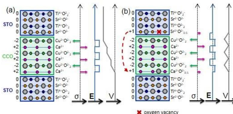
Fig.1 Sketch of CCO/STO SLs. (a) Unreconstructed interfaces with the diverging electrostatic potential. (b) Reconstructed interfaces by oxygen redistribution in the alkaline-earth metal interface planes.
