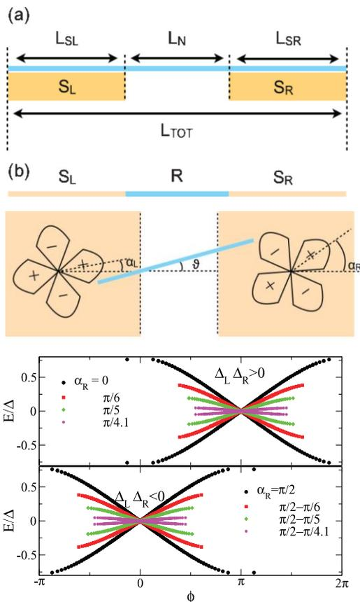
(a) Side view of the superconductor-InAs nanowire - superconductor heterostructure.
