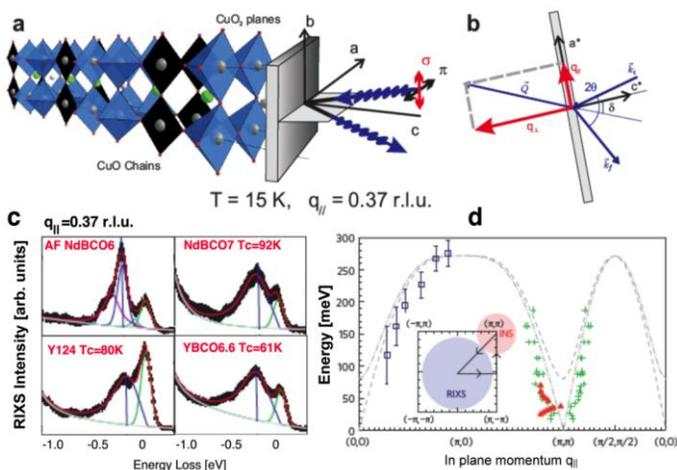
Resonant Inelastic x-ray Scattering reveals charge and spin excitations in cuprates. a) and b) schematics of the RIXS experiment in the case of 123 cuprates. c) RIXS vs energy loss spectra for differently doped cuprates. d) Energy dispersion of magnon excitations obtained from RIXS (open squares) compared to neutron scattering data.
