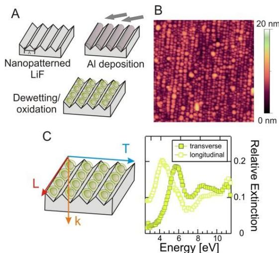
*Fig.1: A: schematic representation of the Al NP array fabrication procedure. B: AFM image of an ultradense array of Al NPs. C: optical geometry for extinction measurements. Extinction spectra measured in longitudinal and transverse optical geometry.*
