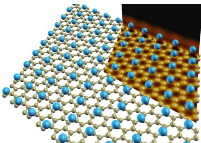
*Lithium adatoms on graphene and charge density of the interlayer state*
