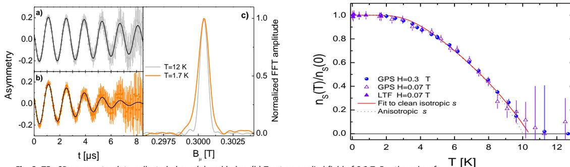
**Fig. 2:** TF- $\mu\text{SR}$  asymmetry data collected above (a) and below (b)  $T_c$  at an applied field of 0.3 T. For the sake of clarity the time-dependent asymmetry is represented in a 40-MHz rotating frame. (c) FFT real amplitude of the data shown in (a) and (b).
