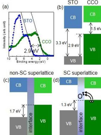
Fig.2 (a) Valence-band spectra for the CCO and the STO. (b)–(d) Schematic diagram of the valence and conducting bands: (b) uncoupled CCO and STO, (c) non-SC SL and (d) SC SL.
