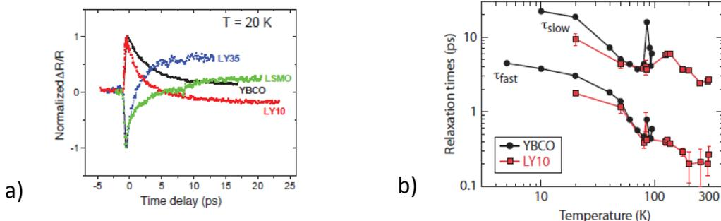
a) Normalized  $\Delta R/R$  transients versus time delay measured at 20 K for our LY10 and LY35 bilayers, as well as the pure YBCO and LSMO reference samples. b) Characteristic fast and slow relaxation times ( $\tau_{fast}$  and  $\tau_{slow}$ ) extracted from the experimental  $\Delta R/R(t)$  plots for our LY10 and pure YBCO samples as a function of temperature.
