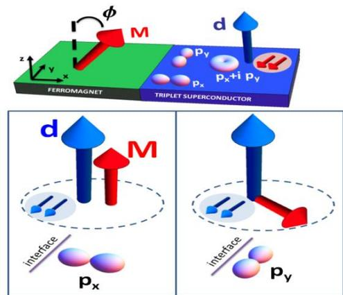
Fig.2: Spin-orbital coupling emerging at the interface of a spin-triplet superconductor with a ferromagnet
