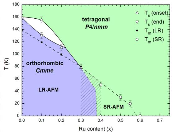
Fig.2: Phase diagram of  $La(Fe_{1-x}Ru_x)AsO$
