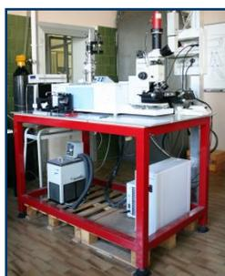
*Interferometer BRUKER 66V for Infrared Spectroscopy equipped with an infrared microscope and a cryogenic apparatus for transmittance and reflectivity measurements down to 5 K.*
