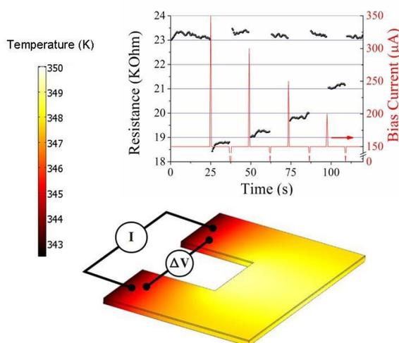
Temperature distribution calculated on a VO<sub>2</sub> / TiO<sub>2</sub> cantilever under 100 µA bias current. Sample temperature is fixed at 343 K and multi-resistance states written by current pulses of different magnitude, cantilever is powered with 150 µA current bias. Erasing is possible by a short pulse to zero.
