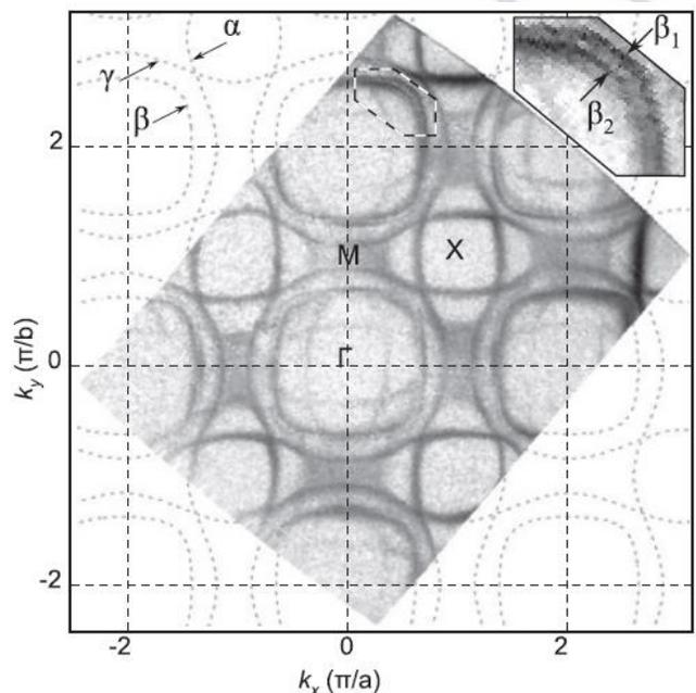
Fig.1: Fermi Surface map of  $Sr_2RuO_4$  as obtained by ARPES measurements where the three bands contributing are observed. The inset shows the splitting of the  $\beta$  band.
