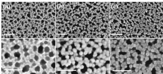
Top-view SEM images of (a) a free PS substrate (interpore spacing 50 nm, pore diameter 15 nm) and Nb nanowire networks deposited on PS with nominal thickness of (b) 3.5 nm, (c) 7 nm. In the upper (lower) panels, the images acquired at lower (higher) magnifications are reported. The white scale bar is 100 nm.
