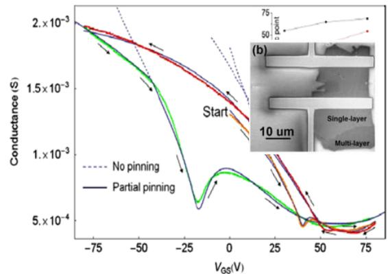
Fig.2 Electrical cycles produce the appearance of two conductance minima. The double dip is the result of a different Fermi level alignment within the graphene at the contacts with respect to the bulk channel .
