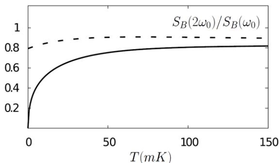
*Temperature evolution of the ratio between the heights of colored noise peaks at the Josephson frequency  $\omega_0$ , of the single quasiparticle  $e/4$  and at frequency  $2\omega_0$  of the double quasiparticle  $e/2$ . The solid line represent the Pfaffian model and the dashed line the anti-Pfaffian model.*
