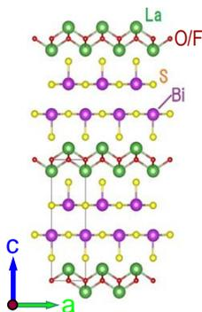
**Fig. 1:** Crystal structure of  $\text{LaO}_{0.5}\text{F}_{0.5}\text{BiS}_2$ ; the solid line indicates the unit cell. (Y. Mizuguchi et al. *J. Phys. Soc. Jpn.* 81, 114725 (2012)).
