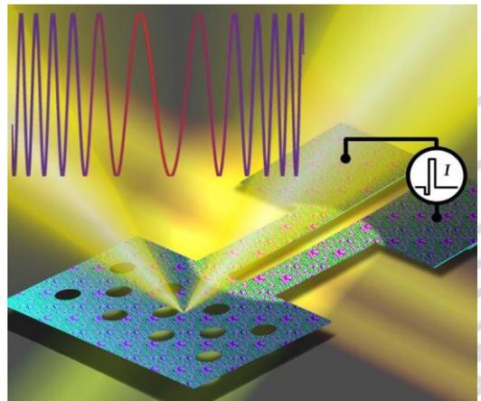
Fig.2: A programmable micromechanical resonator based on a VO<sub>2</sub> thin film. Multiple mechanical eigenfrequency states can be programmed using Joule heating..
