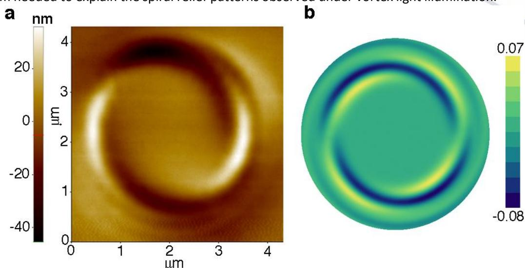
Figure – (a) Relief spiral patterns induced on the polymer by an impinging vortex light beam. (b) Pattern predicted by our model.
