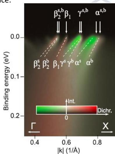
Fig. 2 Circular-dichroic signal to separate the surface and bulk bands in  $\text{Sr}_2\text{RuO}_4$ . In order to facilitate the comparison between the bands exhibiting circular dichroism and those with negligible dichroism, we plot them in this way: the brightness corresponds to the sum of intensities obtained with opposite polarizations (circular right + circular left) and the color, ranging from green through white to red, encodes the dichroism strength (circular right - circular left).
