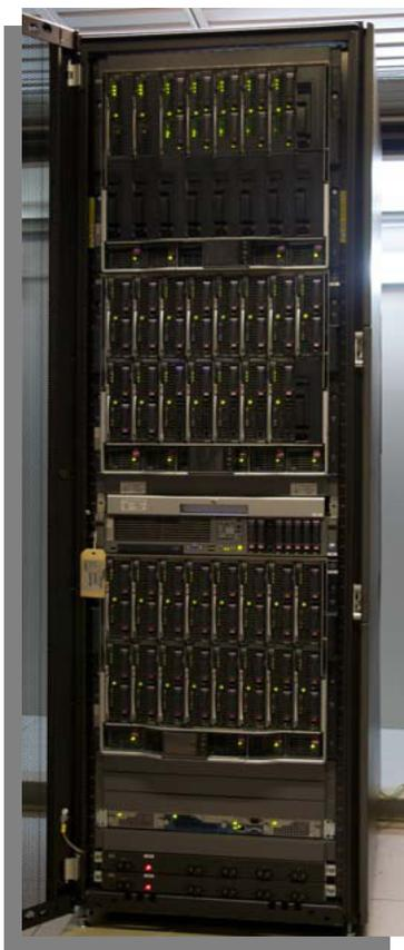
Cluster multiprocessors for advanced computation and high performance made of 38 nodes biprocessors (Intel Xeon with multicore technology, clock from 2.8 to 3.2 GHz), with 8 to 48 GB RAM per node. The overall number of cores and RAM is 200,624 GB. The nodes are connected with Infiniband to have high speed data transfer.
