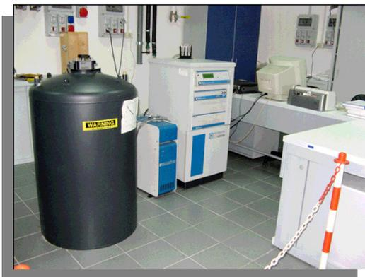
PPMS is a system for modular measurements, that schematically is constituted by a 9 Tesla superconducting magnet, a cryostat for the sample temperature control, electronics needed to manage through PC all present sensors and devices, and a series of interchangeable inserts appropriately designed to measure different physical quantities.
