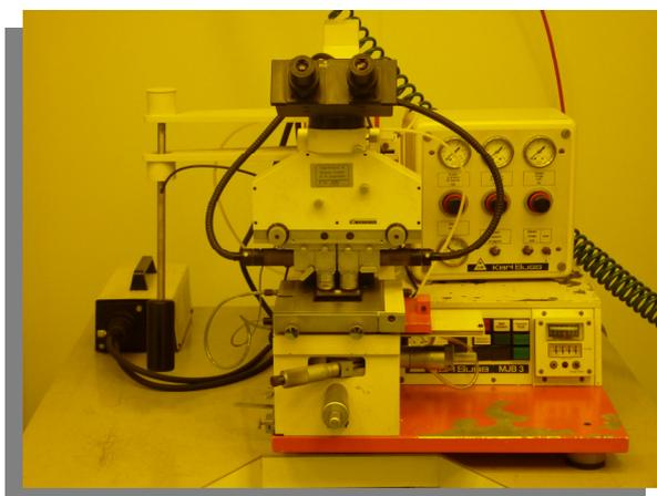
Laboratory dedicated to optic lithography in class 1000 Clean Room, with Mask Aligner Karl Suss with UV lamp, spinner Cammax and spinner Laurell, drying oven, chemical bench, optical transmission and reflection microscope.
