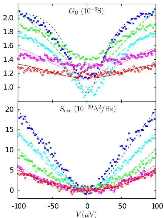
Fit of the experimental data for the conductance (top panel) and noise (bottom panel) taken at Weizmann Institute of Science using our theory"
