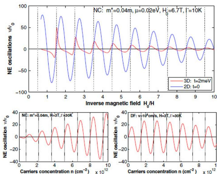
Normalized Nernst-Ettingshausen oscillations in 2D and 3D as a function of the inverse magnetic field and carriers concentration for normal carriers (NC) and Dirac fermions (DF).
