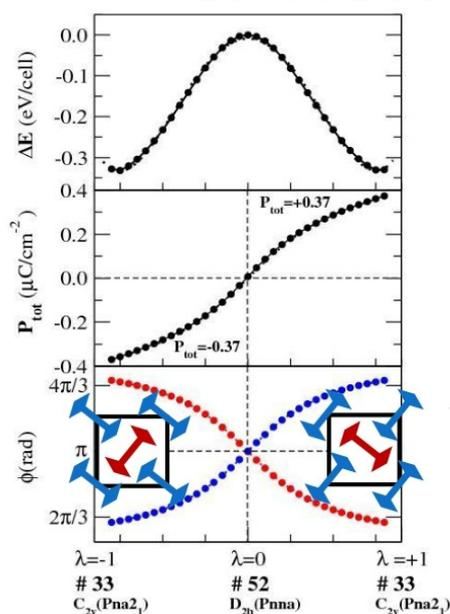
Path connecting the the virtual nonpolar and the two polar phases with opposite polarizations. a) Total energy difference with respect to the paraelectric phase; b) The polarization  $P_{tot}$  as a function of  $\lambda$ ; c) Evolution of the Jahn-Teller phases as a function of  $\lambda$ . Blue and red color refer to the two Cu sublattices with different direction of the elongation axis in the  $ab$  plane.
