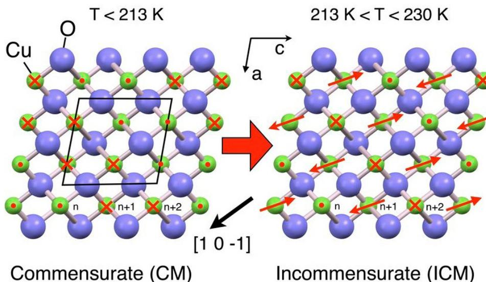
In the ICM phase, the CuO becomes multiferroic, with a finite and switchable Pb along the b axis (Fig. adapted from <http://www.zeitnews.org/>)
