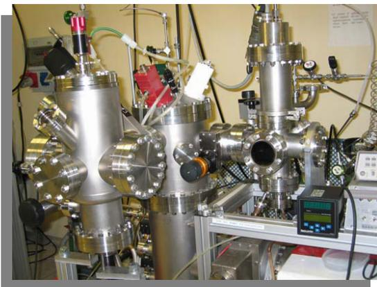
Three chambers ultra-high vacuum system: one of these, equipped with three DC and RF 2.0" sputtering magnetrons, is connected to the other two, both with independent access. The second chamber is equipped with an etching ion gun and a self-made substrate cooling system based on N<sub>2</sub> gas flow, while the third one has a 2" DC and RF sputtering magnetron and a substrate holder with a distance that can be changed without breaking vacuum.
