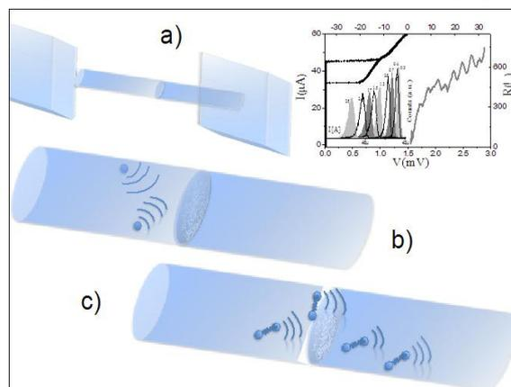
Top right inset: Current-Voltage characteristics. Switching current probability distributions versus bias current for different temperatures down to 300 mK. Resistance versus voltage (voltage scale at the top). a) Scheme of the YBaCuO nanochannel; b) and c) enlargement of grain boundary (GB) region belonging to the nanochannel. Interfering quasiparticles and Cooper pairs transport processes across the GB are sketched in b) and c) respectively.
