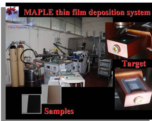
MAPLE (Matrix Assisted Pulsed Laser Evaporation) system for biomaterials and polymeric thin film deposition composed by a vacuum chamber (pressure down to  $10^{-7}$  mbar) and a Qswitched Nd:YAG pulsed (7ns, 0.5-10Hz) laser operating in IR (1064nm, 1.17eV, 500mJ/pulse) VIS (532nm, 2.33eV, 100mJ/pulse) or UV (355nm, 3.49eV, 90mJ/pulse) with in place target refrigeration (liquid nitrogen, 77K) and substrate heating (up to  $\sim 470$ K)
