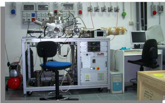
UHV dc magnetron sputtering equipped with a load-lock chamber. The systems has 3 sources, one especially designed for the fabrication of ferromagnetic materials. The deposition chamber is equipped with a movable protecting shutter driven by a pc controlled step motor, in order to fabricate up to 8 samples in the same deposition run. This solution allows the realization of different layered hybrid structures under identical deposition conditions.
