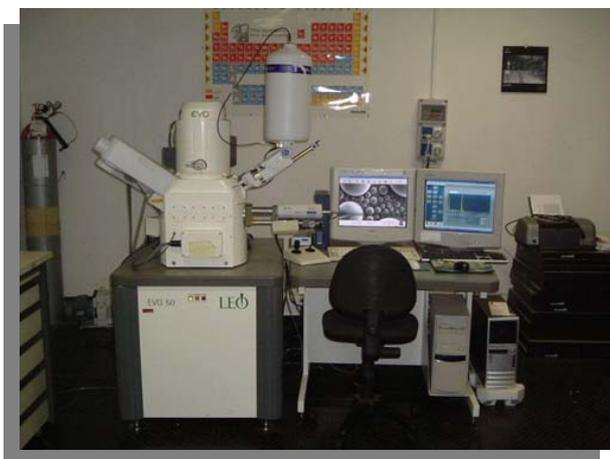
The electron microscopy facility is constituted by a tungsten/LaB6 scanning electron microscope (SEM) (LEO EVO 50) with a secondary electron detector for surface imaging and a 4-quadrant back-scatter electron detector for density imaging detector. The analytical instrumentation is comprised of an Oxford Instruments INCA ENERGY (EDX) xray analysis system, INCA WAVE (WDX) wavelength dispersive x-ray spectrometer and INCA CRYSTAL (EBSD) electron back-scatter diffraction.
