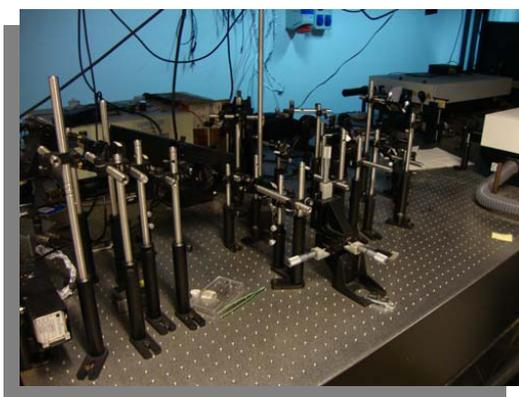
Experimental apparatus for phase-resolved second harmonic generation from surfaces for characterization of surfaces and buried interfaces. The set-up is based on a Nd:YAG laser system delivering pulses of 30 ps of duration at a repetition rate of 10 Hz and energy per pulse up to 60 mJ. The laser is provided with crystals for frequency duplication and triplication.
