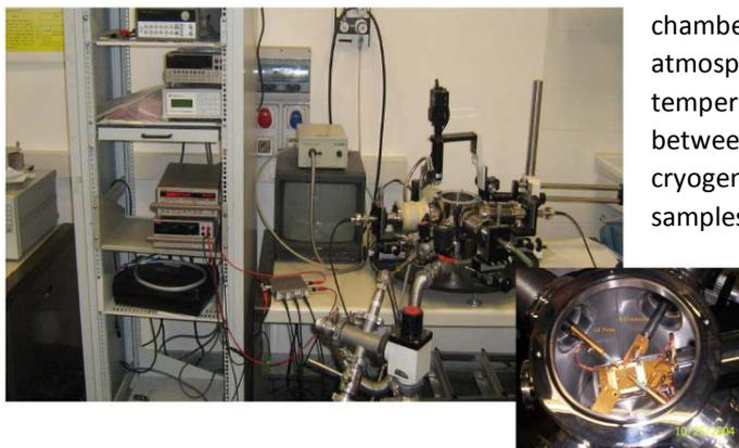
The Probe station system is suited for electrical measurements both in DC and AC regimes (up to 1 MHz). Electrical contacts are realized by three metallic tips mounted on micrometric slides. Probe station is equipped with a vacuum chamber to perform measurements in controlled atmosphere. It is possible to carry out variable temperature measurements in the range between 5K and room temperature by using cryogenic liquids. The temperature of the samples is monitored by two thermometers.
