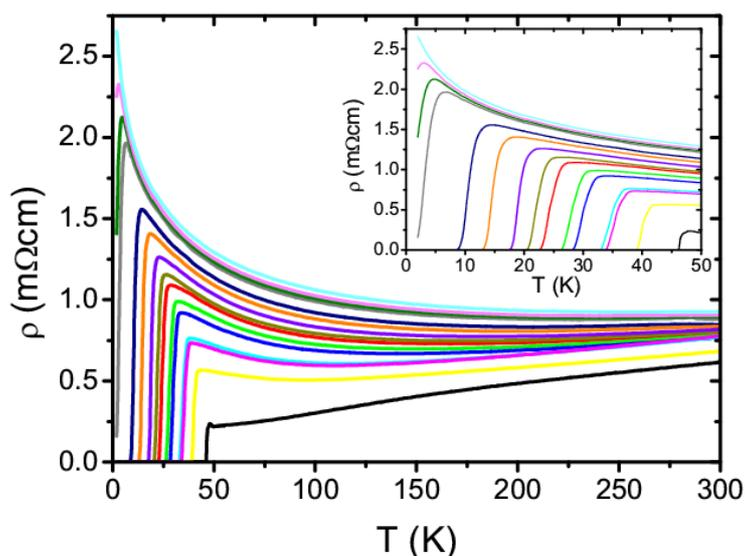
Despite high densities of irradiation defects, the dose at which  $T_c$  is suppressed to zero is comparable to that for MgB<sub>2</sub> but is well above the corresponding values for cuprates. Such remarkably weak  $T_c$  suppression by strong magnetic and nonmagnetic disorder may reveal novel features of superconductivity and magnetism in pnictides.
