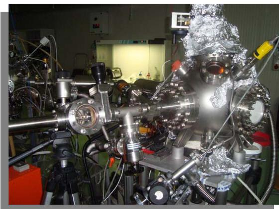
Pulsed laser deposition system Pressure down to  $10^{-11}$  mBar and up to  $10^{-5}$  mBar  $\text{O}_2$ ; substrate temperature up to  $1200^{\circ}\text{C}$ . Fast entry system for sample loading, RHEED; 4 targets; UHV sample manipulation by wooblestick. The system is specifically designed for intermetallic thin films deposition and is interfaced with a cryogenic STM by a UHV transfer chamber.
