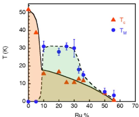
The paper reports on the recovery of short range static magnetic order and on the concomitant degradation of the superconducting state in optimally F-doped  $\text{SmFe}_{1-x}\text{Ru}_x\text{AsO}_{0.85}\text{F}_{0.15}$  for  $0:1 \leq x \leq 0.5$  synthesized at CNR-SPIN. The two reduced order parameters coexist within nanometer-size domains in the FeAs layers and finally disappear around a common critical threshold  $x_c \sim 0.6$ .
