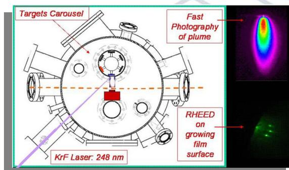
Top view of the deposition chamber and of the two diagnostic tools used for monitoring the plume expansion (ICCD camera) and the film growth (RHEED)
