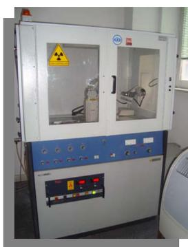
Bragg Brentano diffractometer for powders and thin films. The theta angle movement is independent from 2theta. The setup allows low angle measurements so that it can be used for thin films thickness measurements (range 10-100nm). It mounts  $1^\circ, 1/2^\circ, 1/4^\circ, 1/30^\circ$  slits on the incident beam.  $1^\circ, 1/2^\circ, 1/4^\circ$  slits, Ni filter and graphite monochromator are on the diffracted beam side.
