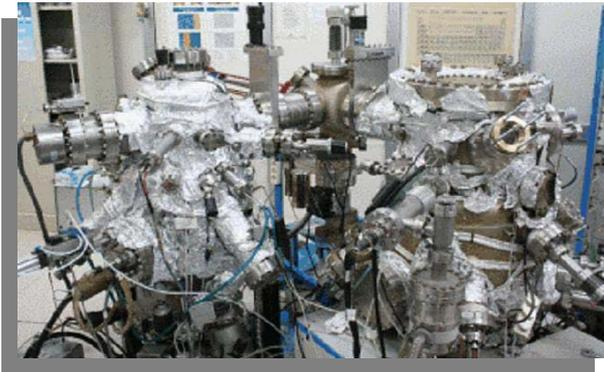
The system consists of a UHV Chamber equipped with different effusive cells inferred (by DCA) to the evaporation of individual materials. The system is equipped with e-gun STAIB for the analysis of in-situ growth (RHEED). It is also equipped with a pre-Chamber for loading the samples without breaking the vacuum conditions in the main Chamber. This last room is also equipped with an independent pumping system.
