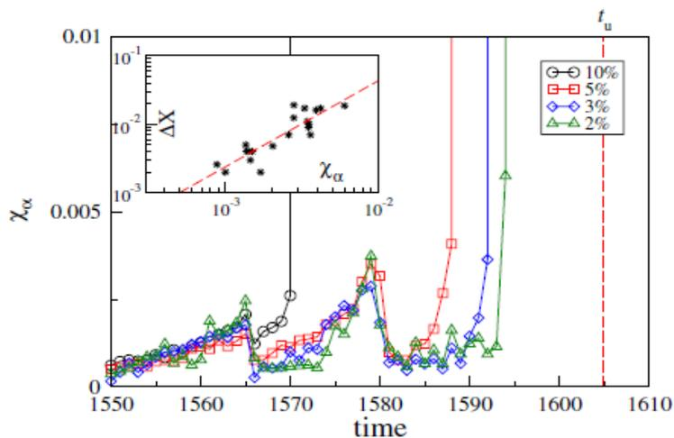
The figure shows the response of the system to perturbations of different intensities, as a function of time, across small and large slips. Before a slip of size  $\Delta X$ , the susceptibility reaches a maximum  $\chi_\alpha$ . The inset illustrates that these two quantities are correlated. This implies that by measuring the system's response to external perturbations it is possible to infer the size of the next slip, i.e. the amount of energy the system will release.
