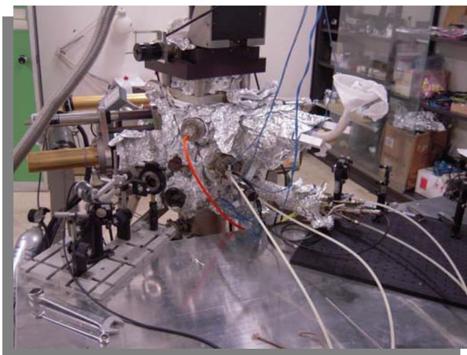
In-situ UHV magneto-optical Kerr effect (MOKE) magnetometer working with laser diodes at 670 and 532 nm. Lock-in detection of the Kerr signal to achieve extreme sensitivity. Longitudinal and polar MOKE configurations can be implemented for the measurement of the in-plane and out-ofplane components of the magnetization. Sample temperature from 130 to 800 K. Maximum magnetic field 1000 Oe.
