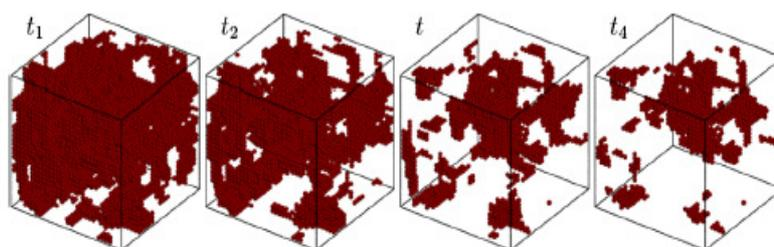
The figure shows the particles of the investigated model system which have not moved in the time interval 0-t. These particles are correlated space over a distance known as the dynamical correlation length. Different theories predict this length to be the one governing the slow dynamics of the system. Our work proved that in this model system this is not the case, and therefore challenges existing theories of the structural glass transition.
