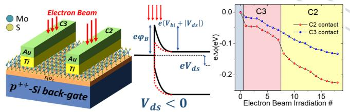
Fig. 1: (a) MoS<sub>2</sub> FET layout. (b) Low-bias energy band diagrams (black) and modification under electron irradiation (red) of contact, resulting in barrier lowering ( $\bar{\varphi}_B$ ). (c) Zero-bias Schottky barrier variation at the contact C2 and C3 as a function of the irradiation number.
