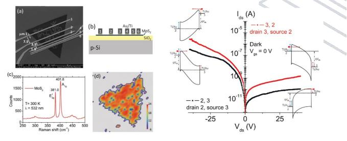
Fig.1: a) SEM top view of a CVD-synthesized bilayer  $MoS_2$  with Ti/Au contacts. b) Schematic of the back-gate transistors. c) Raman spectrum of the bilayer  $MoS_2$ . d) Map of the difference between  $A_{1g}$  and  $E_{2g}$  peaks of micro-Raman spectra.
