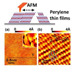
Fig.1: (a) Topography of a PDI8-CN<sub>2</sub> monomolecular terrace revealing an ordered, rippled surface. In the inset, a large-scale morphology (1.5 × 1.5  $\mu$ m<sup>2</sup>) shows connected mesalike grains forming the polycrystalline thin film. (b) High-resolution topography of the periodic surface structure, with superimposed the anisotropic ab unit cell. Ellipses indicate the orientation of the alkyl chains predicted by a bulk structural model.
