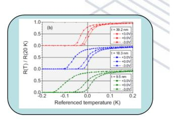
Fig.2: Effect of a gate voltage V<sub>G</sub> =  $\pm 3$  V on the R(T)/R(20 K) vs T curves for three values of thickness: 39.2, 18.3, and 9.5 nm. The referenced temperature is defined as T\* =  $[T-T_c^{ref}]_{VG} - [T_c^{active}-T_c^{ref}]_0$ .
