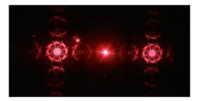
Figure 1. Images generated by the hologram in the visible range. These images were captured by a color chargecoupled device camera
