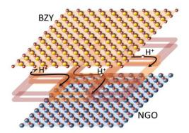
Schematic drawing of the interface between BZY film and NGO substrate with the dislocation network as fast pathway for proton conduction.
