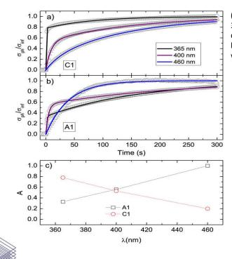
(a) Photoresponse of C1 and (b) photoresponse of A1 at 365 nm (black), 400 nm (red), and 460 nm (green). The data are normalized to the asymptotic value  $\sigma_{inj}$ ; solid lines are fit curves. (c) Dependence of A vs. radiation wavelength  $\lambda$  for both samples.
