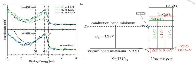
Left image: Resonant photoemission on the Ti 3+ states of the Ti L-edge. The presence of states at the Fermi level, with similar spectral shape, is seen for all samples. Right image: band diagrams are derived from our data.
