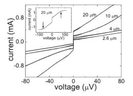
FIG. 1. Current-voltage characteristic of 45° [001] tilt bicrystal GBJs with different sizes measured at T = 4.2 K. In the inset, the IV characteristic of a junction 20  $\mu$ m wide shows peaks due to flux motion.
