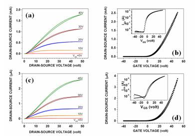
Figure: Output and transfer-curves in the saturation regime measured in vacuum for PDIF-CN<sub>2</sub> transistors fabricated by (a), (b) SuMBD and (c), (d) OMBD techniques on HMDS-treated Si<sup>++</sup>/SiO<sub>2</sub> substrates. In the inset of (b) and (d), semi-log plots of the transfer-curves are shown.
