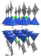
The structure of (YNd)1Ba2Cu3O7 superconductor. Ghiringhelli, G. et al. Science 337, 821–825 (2012)
