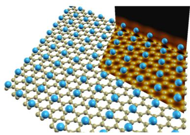
estimated superconducting critical temperature of 18 K when lithium atoms are deposited on both sides of the graphene sheet
