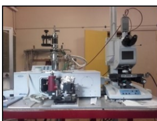
Interferometer BRUKER 66V equipped with a cryogenic apparatus for transmittance and reflectivity measurements down to 5 K and with an infrared microscope Hyperion-II
