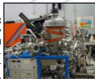
Pulsed Laser Deposition system with in-situ RHEED diagnostics equipped with a multitarget system for oxygen deposition atmosphere enriched with 12% of ozone.
