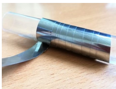
Metallic flexible substrate (INVAR) for the deposition of innovative IBS coated conductors.
