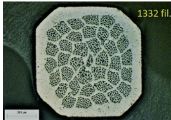
Cross section of a Bi-2212/Ag multifilamentary superconducting wire with 1332 filaments realized within "Alternative HTS wires" project
