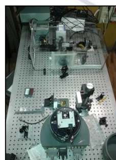
AFM coupled to a Quantum Cascade Laser for infrared microscopy below the diffraction limit.
