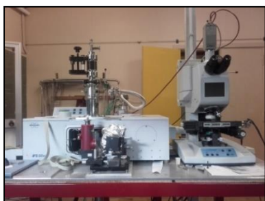
Interferometer BRUKER 66V equipped with a cryogenic apparatus for transmittance and reflectivity measurements down to 5 K and with an infrared microscope Hyperion-II
