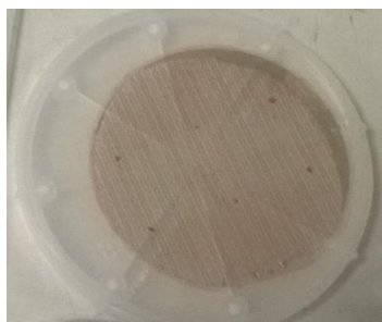
Organic field-effect transistors fabricated on a flexible substrate
