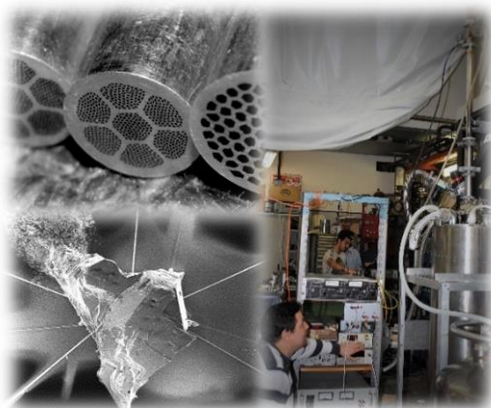
Superconductivity at SPIN: from single crystal to multifilamentary wires for applications. On the right the new cryogenic system at SPIN-GE for high critical current measurements in variable magnetic field and temperature.
