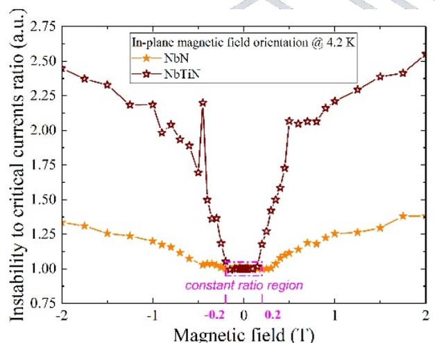
Fig. 2: The ratio  $I^*/I_c$  becomes equal to 1 in the presence of quite low fields for the in-plane orientation. This feature can show up when the thickness is downscaled to few nm, although the width remains of tens of  $\mu\text{m}$ . This ‘*flying bird*’ effect is indeed absent for thicker films.
