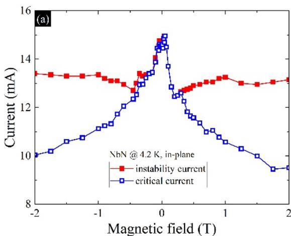
Fig. 1: Instability and critical currents versus magnetic field for the in-plane orientation for NbN sample. This picture reminds a ‘*flying bird*’ and reflects the fact that in the I–V curves there is a threshold field value below which the abrupt jump of vortex instability occurs from the superconducting directly to the normal state.
